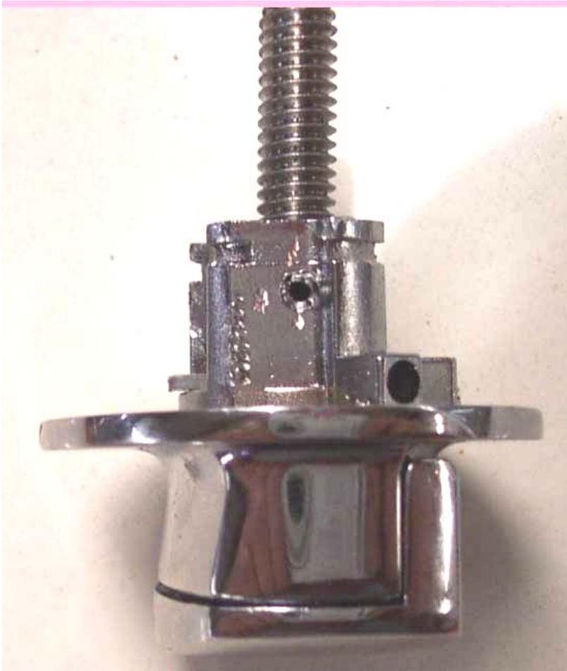
Ok, here it is; install the locking latch and spring, then rest the block and stud between the switch's tabs. Line up the holes, and drive the pin through.
