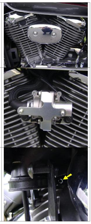
Pull Air Box From the bottom to release the capture post from the rubber grommet seat.
