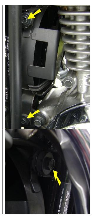
Locate and remove the (1) 10mm bolt on the upper right side of the cooling fan. It is hiding behind the front exhaust pipe.
